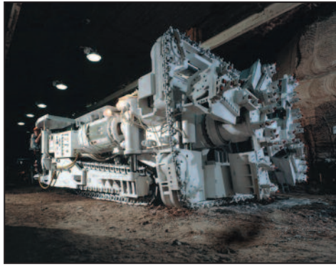
The miner is used to bore into the mine wall to break loose raw ore.
