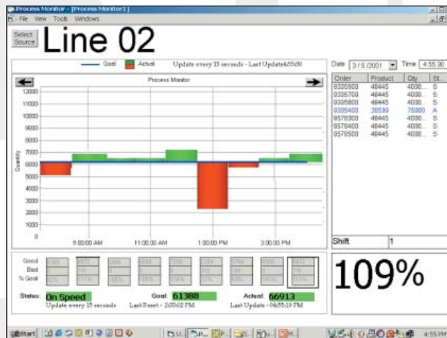
The shop floor control system collects and displays production information as it becomes available. Users are able to review, edit and analyze real time data. Operators are able to see and evaluate their work as it takes place, while supervisors are better equipped to prioritize their time based on what's happening at the moment.
